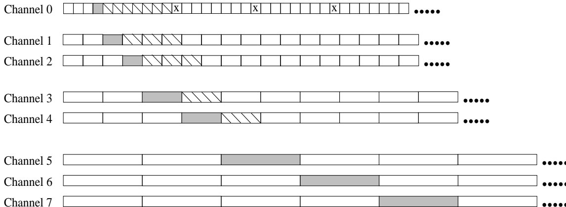
Figure 1. Example Skyscraper Transmission Schedule. ( K = 8 ; W = 8 )
