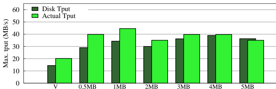
Fig. 14. nginx without Libception using various read_ahead_kb sizes (Linux, WD drive)
