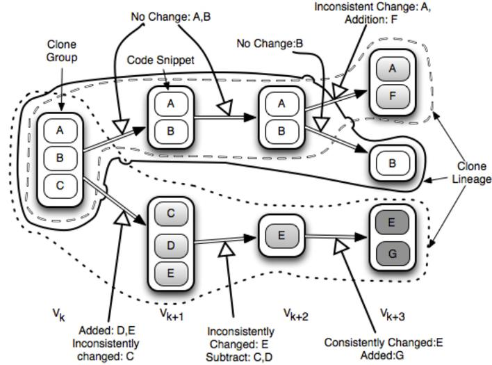
Figure 4: A clone genealogy with two lineages over versions  $v_k$  through  $v_{k+3}$  [201]
