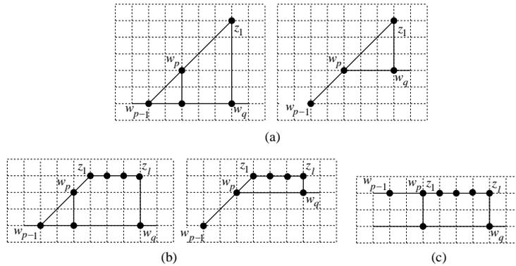
**Figure 6.** Only  $w_q$  has a straight angle. (a)  $|V_k| = 1$ , (b)  $|V_k| > 1$  and the slope of  $(w_{p-1}, w_p) = 1$ , (c)  $|V_k| > 1$  and the slope of  $(w_{p-1}, w_p) = 0$ .
