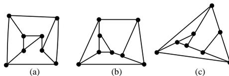
**Figure 1.** (a) A plane graph  $G$ , (b) a convex drawing of  $G$  and (c) a minimum-segment convex drawing of  $G$ .
