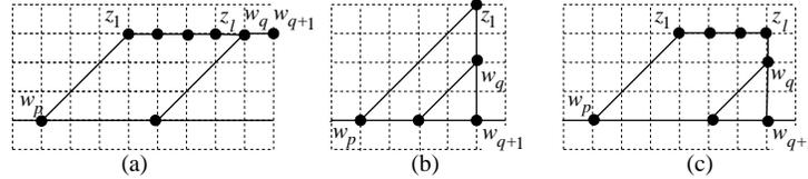
**Figure 7.** Only  $w_p$  has a straight angle. (a) The slope of  $(w_{q+1}, w_q) = 0$ , (b)  $|V_k| = 1$  and the slope of  $(w_{q+1}, w_q) = \infty$ , (c)  $|V_k| > 1$  and the slope of  $(w_{q+1}, w_q) = \infty$ .
