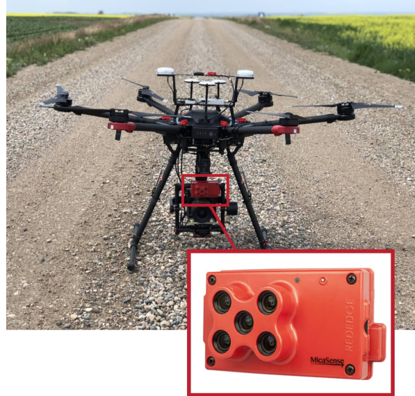
Figure 1: The Micasense Rededge sensor with five separated spectral bands [37] mounted on a UAV.
