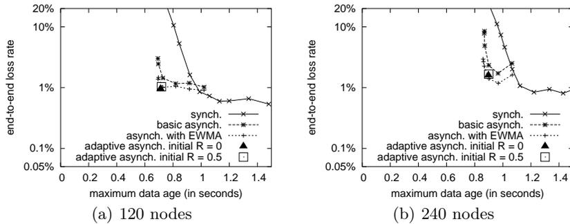
**Fig. 7.** Impact of Number of Nodes (250m x 250m, 20% physical layer loss rate,  $t = 0.5$  sec.)
