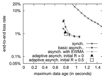
**Fig. 8.** Performance with Clock Shift (clock shift uniform in [-50 ms, 50 ms], 160 nodes, 250m  $\times$  250m, 20% physical layer loss rate,  $t = 0.5$  sec.)
