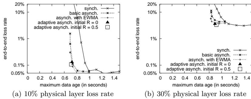
**Fig. 5.** Impact of Physical Layer Loss Rate (160 nodes,  $250\text{m} \times 250\text{m}$ ,  $t = 0.5$  sec.)
