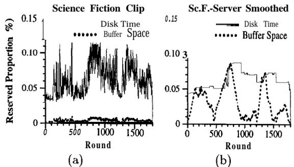
Figure 3: Example of applying the Server Smoothing algorithm. We depict the disk time and buffer space proportion in the system (a) before, and (b) after applying Server Smoothing. The maximum disk time proportion drops from 11.5% to 8.7%, while the maximum buffer space proportion increases from less than 1% to 8.7%. The Seagate Cheetah disk parameters are assumed and server buffer of 256 MB per disk.
