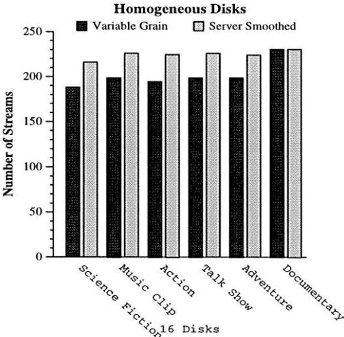
**Figure 5:** The advantage of *Server Smoothing* when applied to Variable Grain Striping can exceed 15% (Action) depending on the stream type. The load was set to 90% on sixteen disks and 256 MB per disk were assumed.
