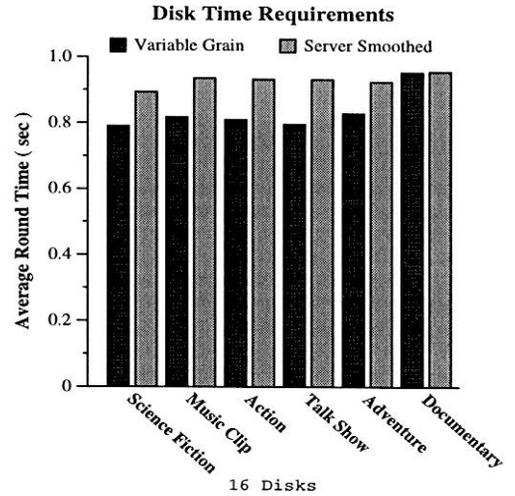
**Figure 6:** With sixteen disks and 90% system load, the average disk time reserved each round increases from less than 80% to over 90% with *Server Smoothing* and server buffer 256 MB per disk. Although the disk time shown corresponds to one of the disks (Disk 0) it was similar (typically within 2%) across the disks of the array.
