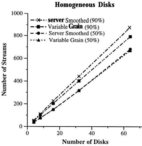
**Figure 4:** With the mixed workload and Variable-Grain Striping (with/without *Server Smoothing*), the sustained number of active streams increases almost linearly with the number of disks. Although at system load 50% all the submitted streams are accepted, at load 90% *Server Smoothing* increases the number of active streams by about 10%. This benefit is maintained across different numbers of disks.
