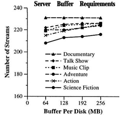
**Figure 7:** With buffer space (per disk) set to 64 MB, more than half of the total benefit of *Server Smoothing* can be achieved (see also Figure 5). Increasing the buffer space to 256 MB farther improves the number of streams in Science Fiction and Action types although at a diminishing degree.
