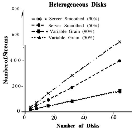
Figure 9: With the mixed workload and plain Variable-Grain Striping, the sustained number of active streams remains the same as the load is raised from 50% to 90%. Instead, when Variable-Grain Striping is combined with Server *Smoothing* the number of streams increases by a factor of 2 at 50% and more than a factor of 3 at 90% load, when compared to that achieved by plain Variable-Grain Striping. Server buffer space of 256 MB per disk has been assumed.
