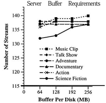
Figure 12: With the server buffer (per disk) set to 64 MB, most of the benefit of *Server Smoothing* can be attained (see also Figure 10). Increasing the server buffer from 64 MB to 256 MB increases only marginally (less than 5%) the sustained number of active streams.
