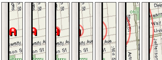
Figure 3: As this location is panned out of the display window, a ring emerges from its center. The ring grows as the location is panned further away.
